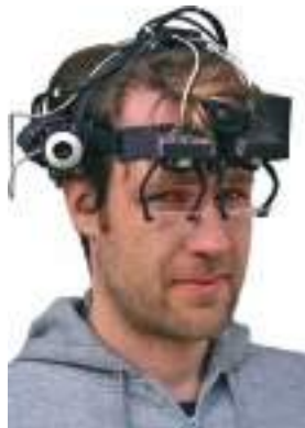
The EyeSeeCam, developed in collaboration with Stefan Glasauer 5 , records eye and head movements and uses this information to steer a camera sitting at the side of the device. In this way, the experimenter can “see through the subject’s eyes”.
