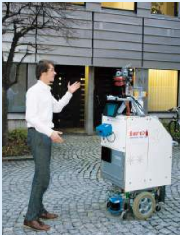
The robot “iuro” interprets gestures and spoken hints by passers-by to find its way.
